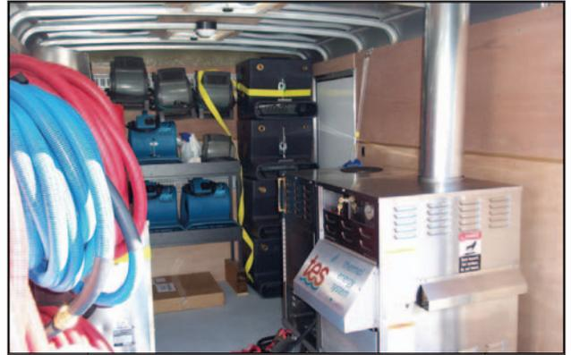
**Ventilation: Two roof vents, 14" x 14"**—Allows for hot air to escape. Roof vents must be open any time TES is running.
