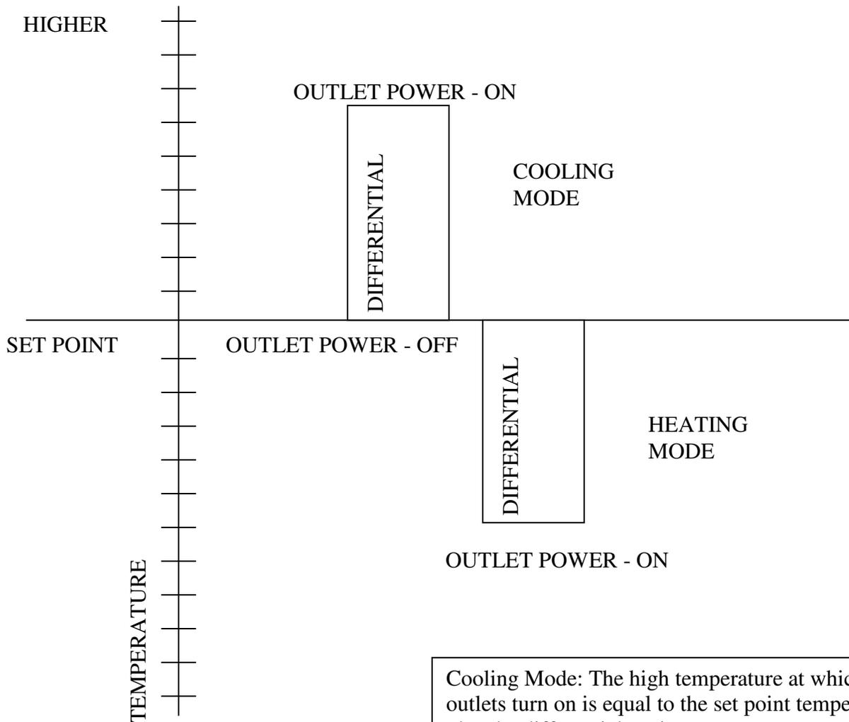
Cooling Mode: The high temperature at which the outlets turn on is equal to the set point temperature plus the differential setting.
