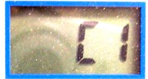
(Our normal use is in the cooling mode. In the heating mode the differential setting is below the set point, meaning that the outlets will turn on when the room temperature is cooler than the set point by the number of degrees at which the differential is set. If the set point is 74°F and the differential is set at 5. The outlets will turn on when the room temperature reaches 69°F. The outlets will turn off when the room temperature returns to 74°F.)
