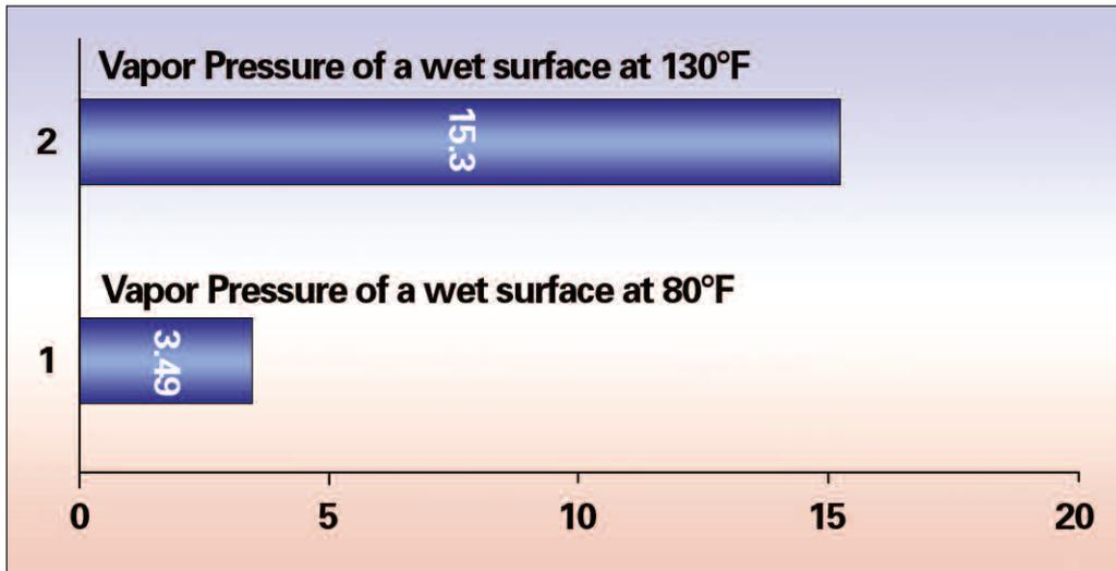
Vapor pressure measured in kPa
